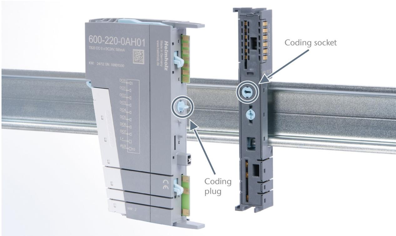
The coding plug and coding socket can each be in one of eight different positions. Each of these eight positions can be used for a specific type of module (Digital In, Digital Out, Analog In, Analog Out, Power). It will only be possible to plug an electronic module into a base module if the position of the coding plug and the position of the coding socket match. If the positions differ, the electronic module is mechanically blocked.
