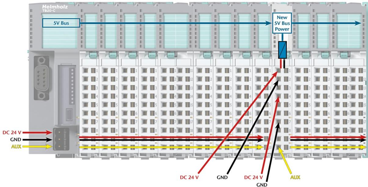
The order no. for the power module is 600-700-0AA01. The electronic module of the power module is light gray like the front connector. The base module of the power module is light gray with a dark top part.
