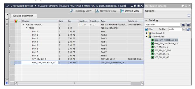
If the Helmholz SFP modules are configured, the FLEXtra PROFINET switch checks whether exactly the configured SFP module has been plugged into the specified port. If an SFP module is missing or an SFP module of a different type is plugged, a diagnosis is triggered. Thus a wrong configuration or a wrong cabling can be detected easily.
