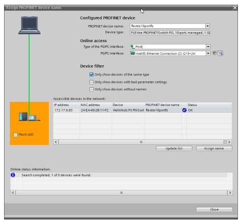
The clear identification of the FLEXtra PROFINET switch is ensured here by the MAC address of the device. The MAC address of the device can be found on the device front of the FLEXtra PROFINET switch.
