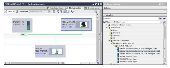
By calling up the object properties, you must give the FLEXtra PROFINET switch a unique PROFINET name in the project and check the IP address for plausibility.
