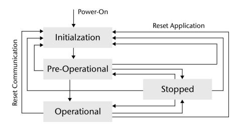
With the NMT command "Operational" [COB-ID:  $000_{hex}$  / data (2 bytes):  $01_{hex}$  node ID], a CANopen device can be switched to the operational status. Once in the Operational state, the coupler's process data will be enabled (RPDO/TPDO communications will be running). The options available for making changes to SDOs may be limited.
